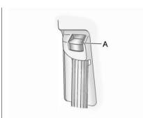
To move it down, push down on the button (A) and move the height adjuster to the desired position. You can move the height adjuster up by pushing up on the shoulder belt guide.
